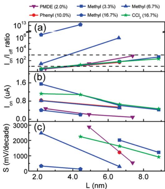
**Figure 6.** (a)  $I_{on}/I_{off}$  ratios, (b) on-state currents, and (c) subthreshold swings of the typical functionalized (5,5) SWCNT FETs at  $V_{bias} = 0.02$  V as a function of the channel length ( $L$ ).
