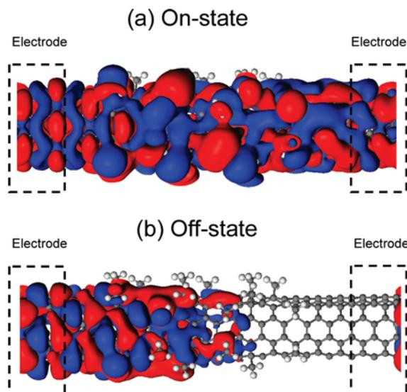
**Figure 7.** Transmission eigenchannels of the (5,5)+methyl(16.7%) FET with a channel length of  $L = 2.21$  nm at the Fermi level for the (a) on- and (b) off-state. The isovalue is  $10^{-2}$  a.u. Red and blue are used to indicate the positive and negative signs of the wave functions, respectively. Gray ball, C; white ball, H.
