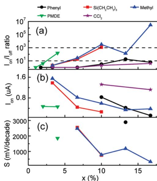
**Figure 4.** (a)  $I_{\text{on}}/I_{\text{off}}$  ratios, (b) on-state currents, and (c) subthreshold swings of the functionalized (5,5) SWCNT FETs at  $V_{\text{bias}} = 0.02$  V as a function of the coverage concentration ( $x$ ). The channel length is  $L = 2.21$  nm for phenyl,  $\text{Si}(\text{CH}_2\text{CH}_3)_3$ , methyl, and  $\text{CCl}_2$  addition, and  $L = 2.46$  nm for PMDE addition.
