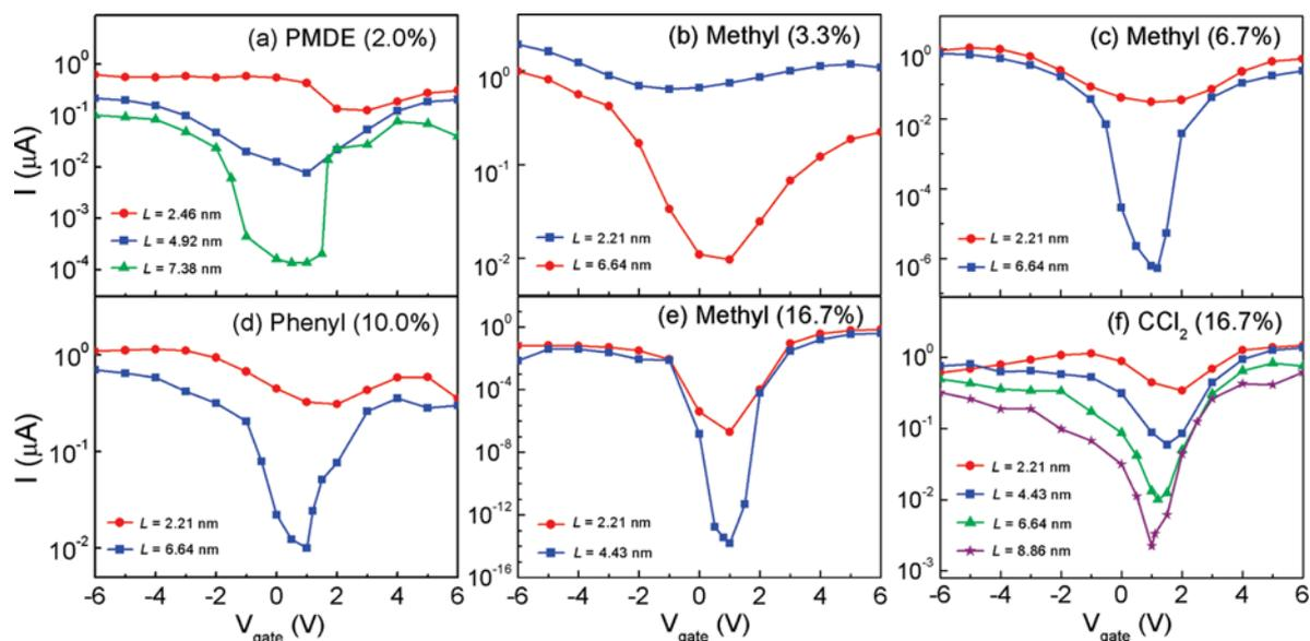
**Figure 5.** Calculated transfer characteristics ( $V_{\text{bias}} = 0.02$  V) of the typical functionalized (5,5) SWCNT FETs as a function of the channel length ( $L$ ).
