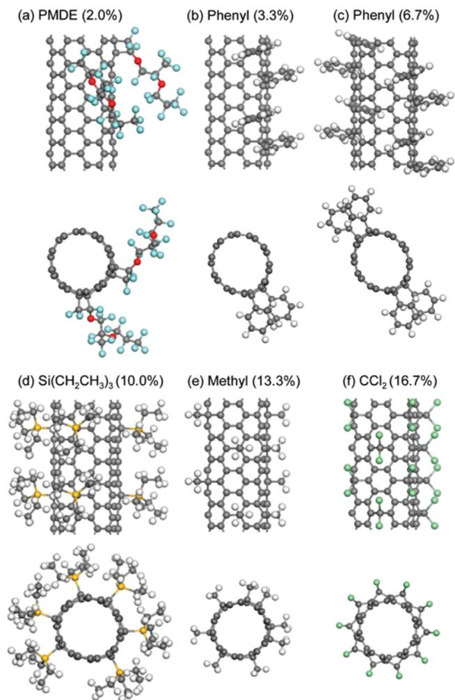
**Figure 1.** Side and top views of the typical optimized infinite functionalized (5,5) SWCNTs in the most stable adsorption configurations. Gray ball, C; white ball, H; yellow ball, Si; red ball, O; blue ball, F; green ball, Cl.
