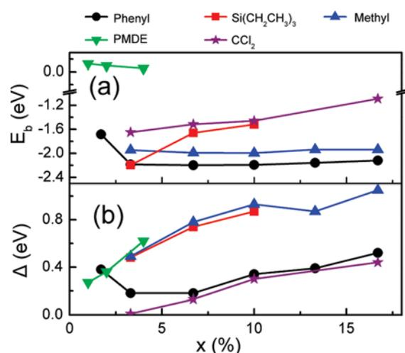
**Figure 2.** (a) Binding energy per radical and (b) band gaps of the infinite functionalized (5,5) SWCNTs in the most stable adsorption configurations as a function of the coverage concentration ( $x$ ).
