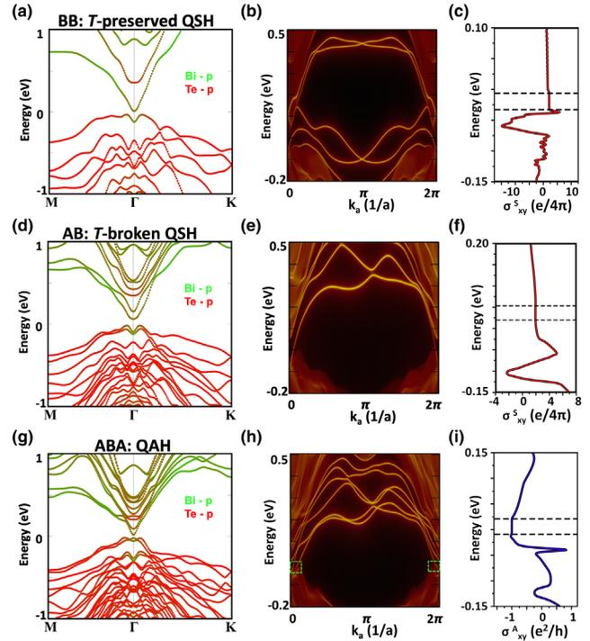
FIG. 3. (a)–(c) Band structure with projection onto different atomic orbitals (a), edge states (b), and quantized spin Hall conductance (c) of *BB* (bilayer Bi<sub>2</sub>Te<sub>3</sub>) configuration. (d)–(f) Same as (a)–(c) but for the *AB* configuration. (g), (h) Same as (a), (b) but for the *ABA* configuration. (i) Quantized anomalous Hall conductance of the *ABA* configuration.
